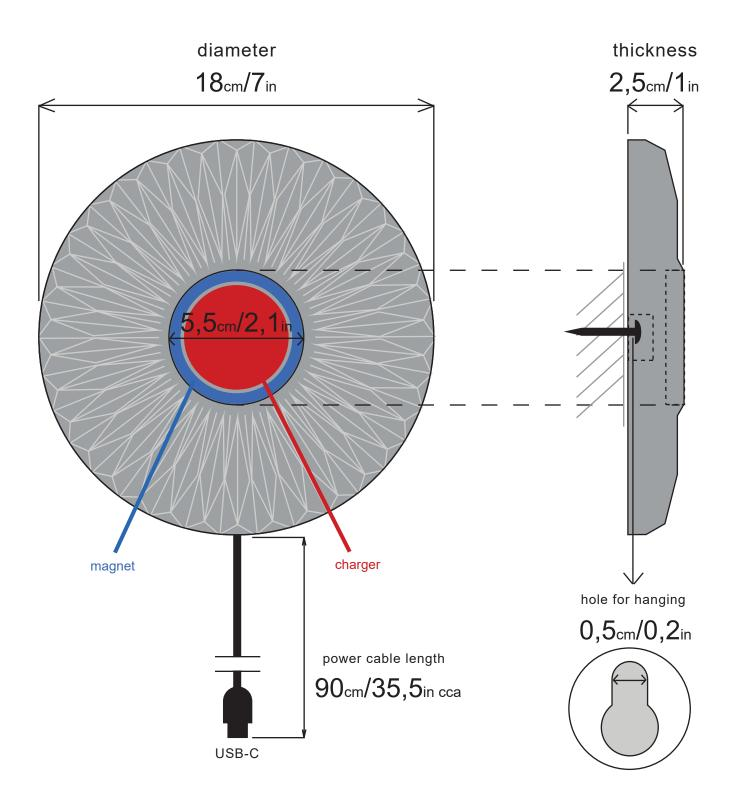
the cable can be routed from side or from below
